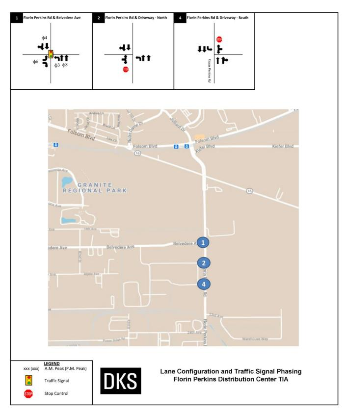
FIGURE 5. INTERSECTION LANE CONFIGURATION AND TRAFFIC SIGNAL PHASING
