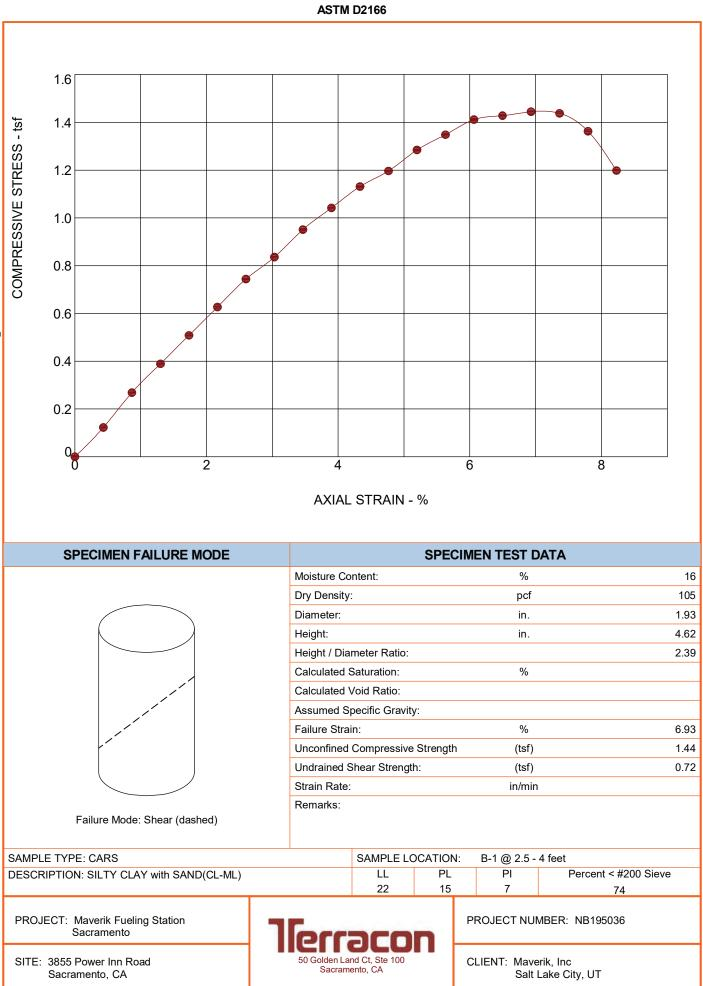
LABORATORY TESTS ARE NOT VALID IF SEPARATED FROM ORIGINAL REPORT. UNCONFINED NB195036 MAVERIK FUELING STATION - SACRAMENTO.GPJ TERRACON\_DATATEMPLATE.GDT 5/22/19
