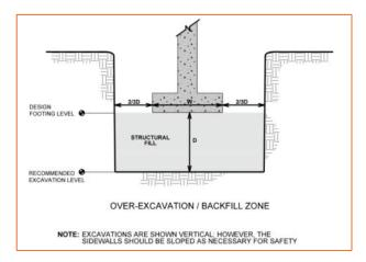
To ensure foundations have adequate support, special care should be taken when footings are located adjacent to trenches. The bottom of such footings should be at least 1 foot below an
