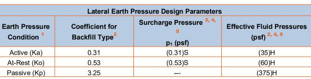
1. For active earth pressure, wall must rotate about base, with top lateral movements 0.002 H to 0.004 H, where H is wall height. For passive earth pressure, wall must move horizontally to mobilize resistance.
