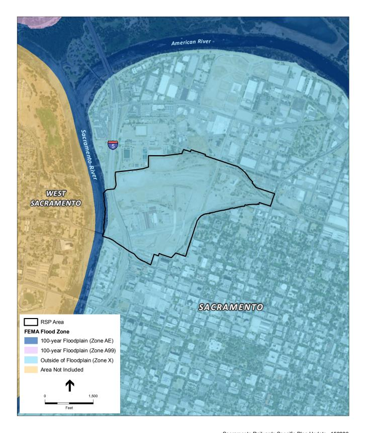
North B Street, was once considered a flood prevention facility, but was never certified or constructed under federal standards to serve as a legitimate flood protection levee. FEMA had credited this structure, along with the UPRR tracks embankment, with providing added protection from flooding for areas within the RSP Area, as evidenced on the current FEMA floodplain map.
