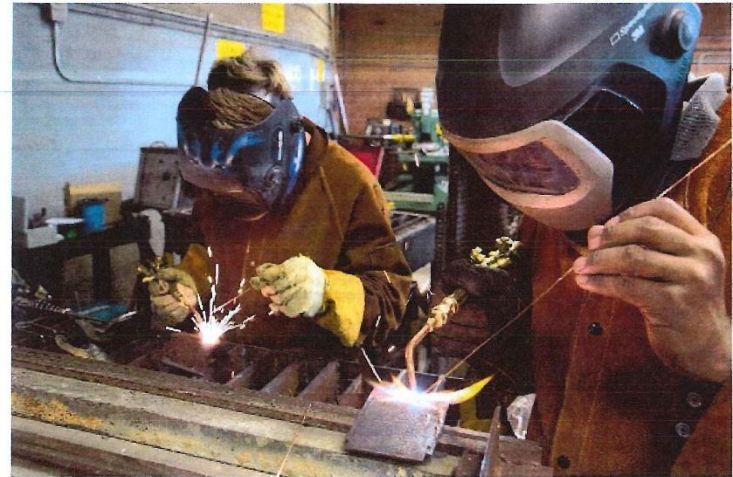
Anatoly Lukavenko, left, and Ritesh Narayan practice oxy-acetylene welding as part of the welding technology program at American River College.
