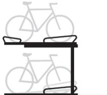
Typically used for high-density indoor parking. Performance varies widely. Models for public use include lift assist for upper-tier parking. Recommend testing before purchasing. Creates safety concerns not inherent to on-ground parking, and requires maintenance for moving parts.
