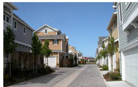
Well-designed alleys provide alternative access to homes and reduce the number of curb cuts, driveways, garage doors, and associated pedestrian/automobile conflicts along street frontages.
