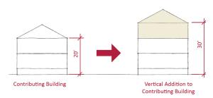
Figure 171. Additions should not cause a building's height to exceed 150% of its historic height.
