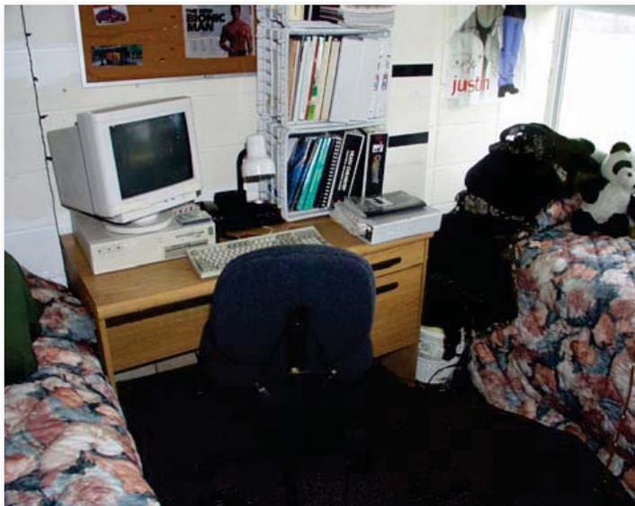
These post-fire photographs of dorm rooms show the difference a sprinkler makes. There is little visible damage in the top photo that had a sprinkler in the room; there was no sprinkler in the dorm room in the bottom picture. The dormitory burn experiment was conducted by the National Institute of Standards and Technology (NIST) and the USFA.
